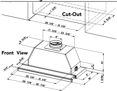
Note: The Cristal HC comes standard in the top vent position. The direct rear vent position can be achieved by rotating the blower housing.
